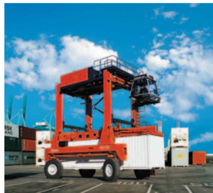
The key to the success of the Shuttle Carrier®, the so-called one-over-one design, is its ability to operate independently, leading to a more efficient work cycle.
