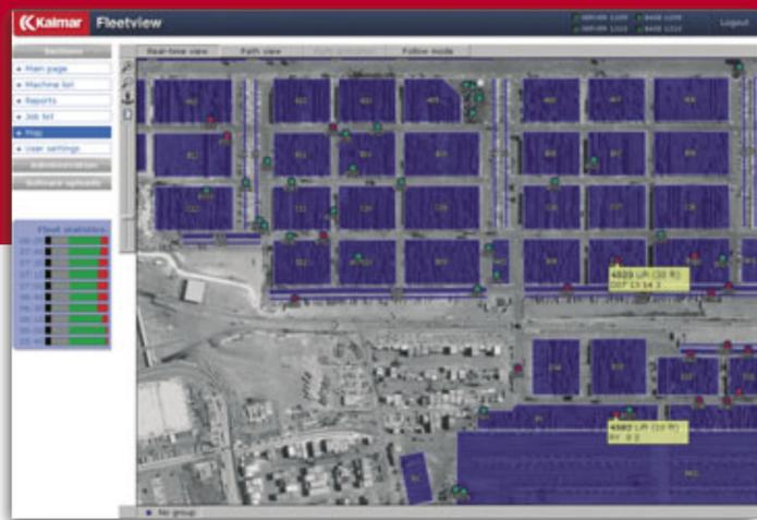
staff to monitor the real-time positioning and efficient control of each machine. Container handling tasks can be assigned to the unit best suitable for the job, thus minimising unladen travelling distances and resulting in better productivity. For a major multi-million TEU terminal operator like Maher, this offers substantial operating benefits.
