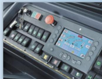
tegrates all functions in a single system and shows full operational and service data on one display panel, makes tractor operations faster, safer and simpler. Its diagnostic capabilities also assist in service and maintenance planning, saving time, effort and cost.
