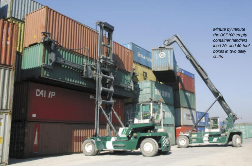
Minute by minute the DCE100 empty container handlers load 20- and 40-foot boxes in two daily shifts.
